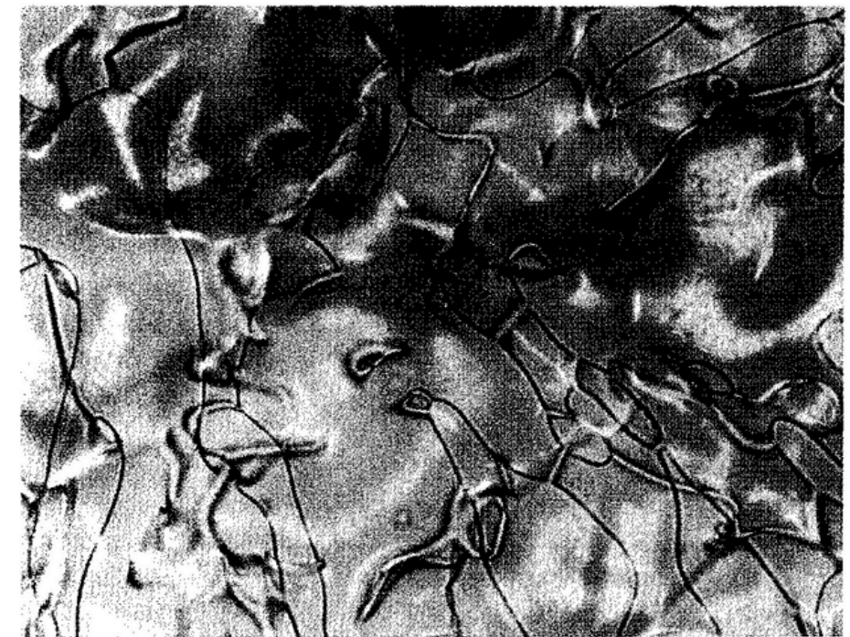
Optical microscope photograph of liquid crystal following temperature quench (Chuang et al. 1991)
