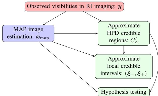
Fig. 2. UQ methodology II: procedure based on MAP estimation [2].
